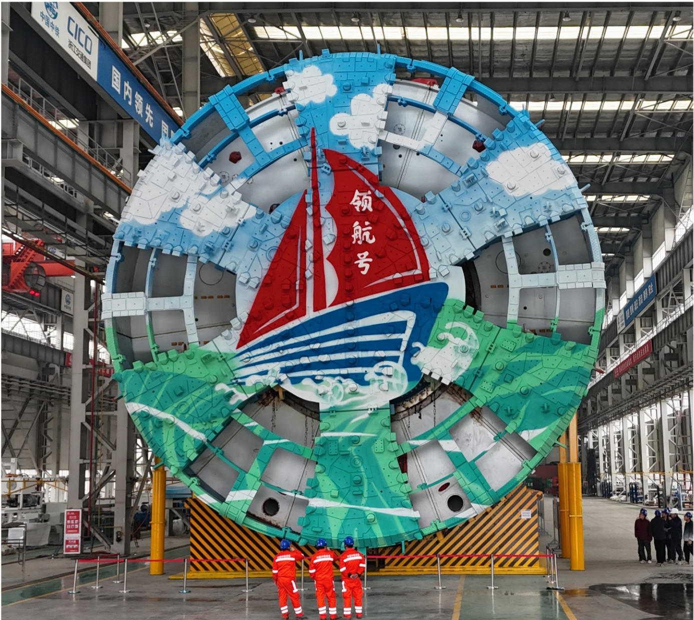
TBM Factory Acceptance Test
