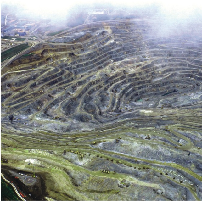
Construction of the roadway faces challenges of large slope and small curve radius.
