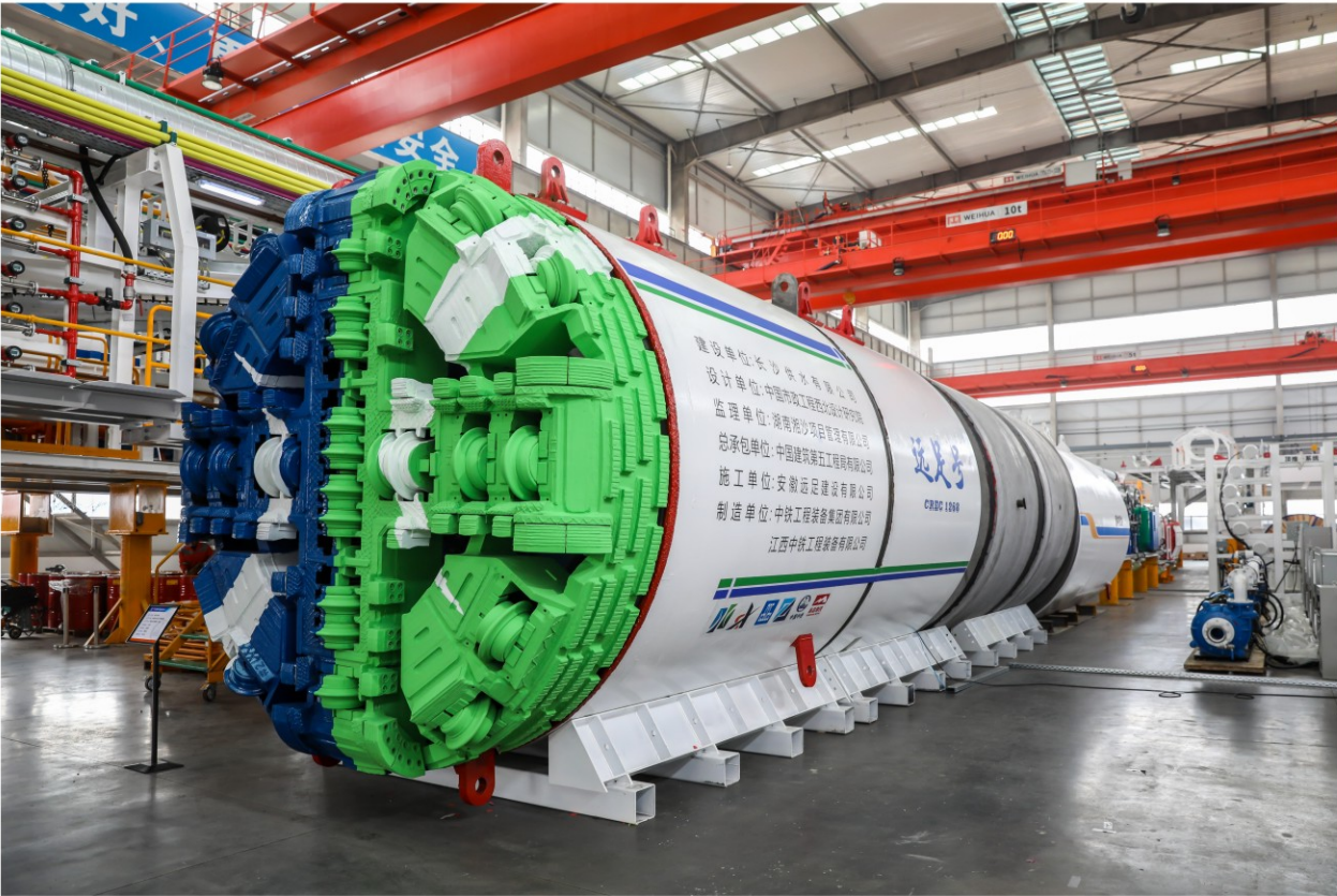
Pipe jacking shield machine "CREC 1268" rolled off the production line.
